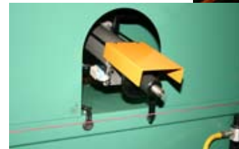
Manual adjustment for the bending roll position.
