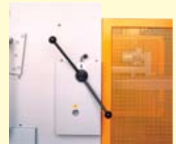
Rapid, single-point, blade gap adjustment device.
