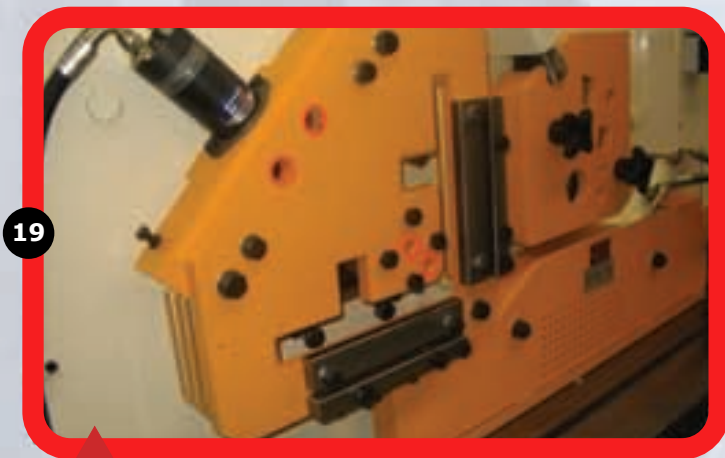
Hydraulic clamps for angle and plate
