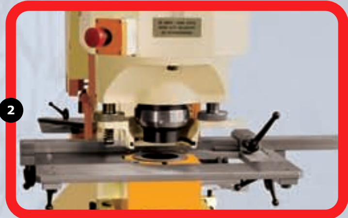
4" Oversize punching unit mounted on machine
