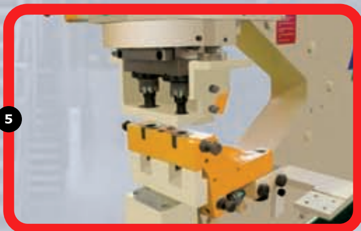
Double punching on gooseneck-type die holder
