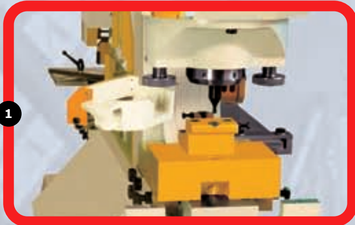
Punching on wing and core section L 1 1/2" to 3".
