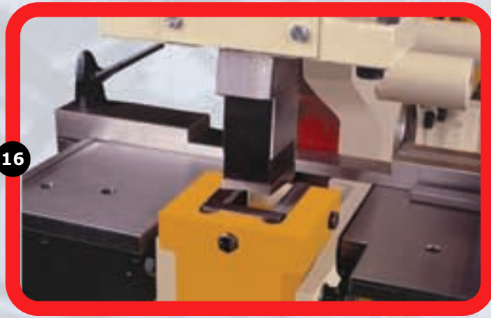
Notching tool mounted at punch end of microcrop
