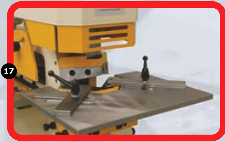
Triangular notching tool with table
