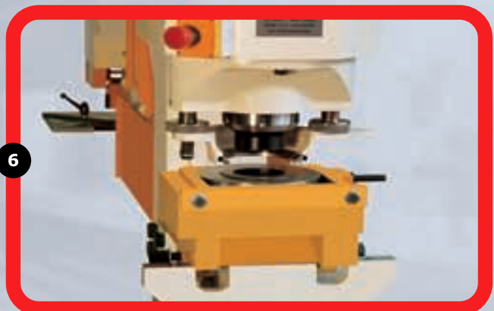
6" Oversize Punching unit mounted on machine.
