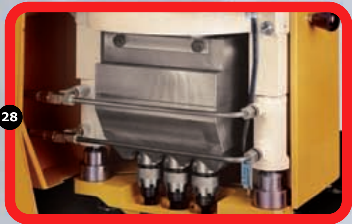
Triple punching with hydraulic stripper
