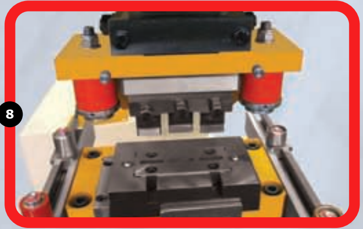
Triple punching 3 holes per stroke with neoprene stripper
